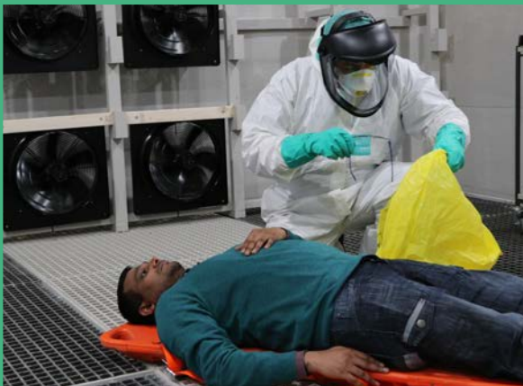
Evaluation of PPE while performing physical tasks within a salt nanoparticle environment.
